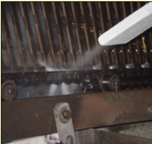
Dry ice blast cleaning of a moving oven chain
